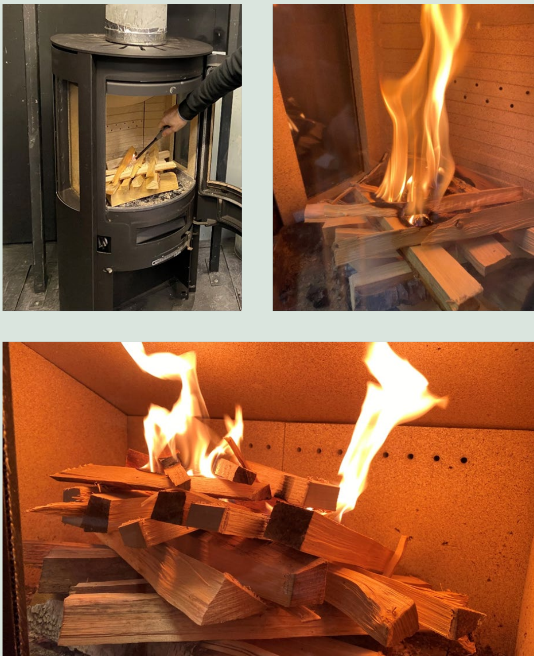
FIGURE 4. Correct positioning of firewood logs and ignition technique. Top: small and medium sized stoves, bottom: large stoves.
