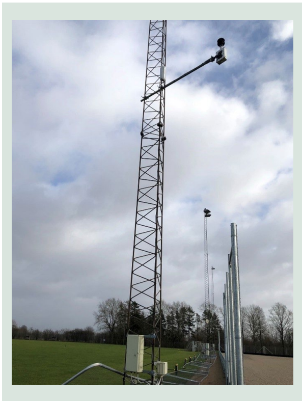
FIGURE 11. The sensor for qualification of background concentration (A5) was located on a mast in the area of Mårslet school.
