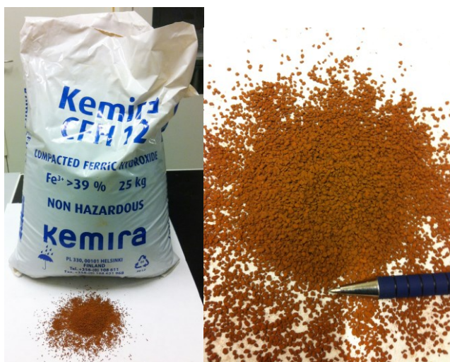
Figur 4-1 Granulat fra Kemira A/S (Compacted Ferric Hydroxide, CFH 12).
